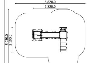
Lenght: 2 820 mm Width: 2 100 mm Height: 2 150 mm
