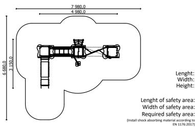
4 980 mm Lenght: Width: 3 150 mm Height: 2 780 mm
