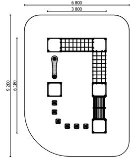
Lenght: 6 180 mm Width: 3 800 mm Height: 1 500 mm
