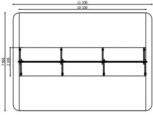
Lenght: 10 330 mm Width: 2 305 mm Height: 2 600 mm
