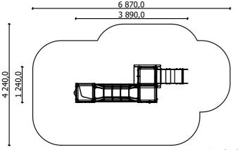
Lenght: 3 890 mm Width: 1 240 mm Height: 1 980 mm
