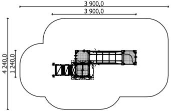
Lenght: 3 900 mm Width: 1 240 mm Height: 2 065 mm
