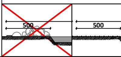
Foundation should be accessible for maintenance.
