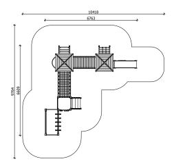
Lenght: 6 763 mm Width: 6 609 mm Height: 3 180 mm
