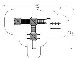
Lenght: 9 144 mm Width: 6 259 mm Height: 3 980 mm
