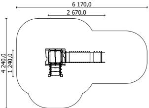
Lenght: 2 670 mm Width: 1 240 mm Height: 2 950 mm 6 170 mm Lenght of safety area: 4 240 mm Width of safety area: 24 m<sup>2</sup> Required safety area: (Install shock absorbing material according to EN 1176:2017)
