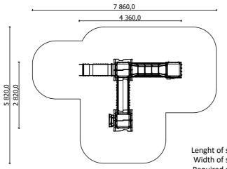
Lenght: 4 360 mm Width: 2 820 mm Height: 2 550 mm
