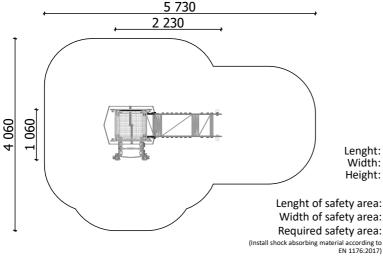
2 230 mm Lenght: Width: 1 060 mm Height: 2 465 mm
