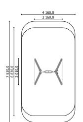
Playground equipment steel foundation is concreted in the ground at the planned location. The equipment can be used after two days when the concrete becomes solid. During assembly no children are allowed in the area.
