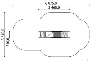
Lenght: 2 465 mm Width: 510 mm Height: 1 620 mm
