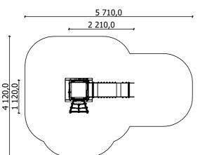
Lenght of safety area: 5 710 mm 4 120 mm Width of safety area: 20 m<sup>2</sup> Required safety area: (Install shock absorbing material according to EN 1176:2017)
