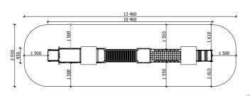
10 460 mm Lenght: Width: 930 mm Height: 1 770 mm
