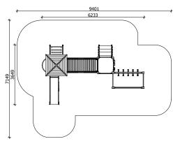
Lenaht: 6 233 mm Width: 3 649 mm Height: 3 180 mm
