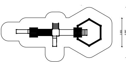
Lenght: 11 600 mm Width: 3 850 mm Height: 3 050 mm
