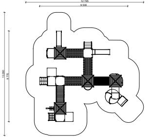
Lenght: 9 530 mm Width: 9 770 mm Height: 3 980 mm
