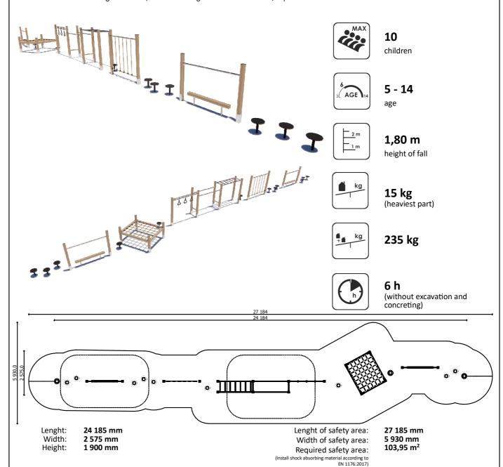
Playground equipment steel foundation is concreted in the ground at the planned location. The equipment can be used after two days when the concrete becomes solid. During assembly no children are allowed in the area. Foundation should be accessable for maintenance.
