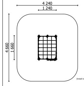
Lenght: 1 240 mm Width: 1 660 mm Height: 1 560 mm
