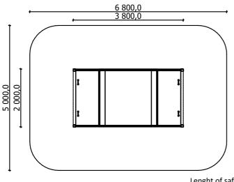
Lenght: 3 800 mm Width: 2 000 mm Height: 0,290 mm
