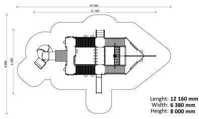
Lenght of safety area: 15 340 mm Width of safety area: 9 880 mm Required safety area: 90,88 m<sup>2</sup>
