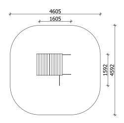
Lenght: 1 605 mm Width: 1 592 mm Height: 1 950 mm
