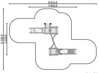
Lenght: 4 820 mm Width: 3 220 mm Height: 2 780 mm
