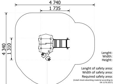
Lenght: 1 735 mm Width: 1 310 mm Height: 2 075 mm
