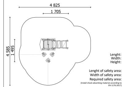
Lenght: Width: 1 705 mm 1 495 mm Height: 2 055 mm Lenght of safety area: 4 825 mm 4 585 mm Width of safety area: 16,95 m<sup>2</sup> Required safety area:
