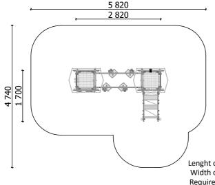
Lenght: 2 820 mm Width: 1 700 mm Height: 1 985 mm
