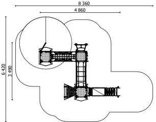
Lenght: 4 860 mm Width: 3 490 mm Height: 2 785 mm
