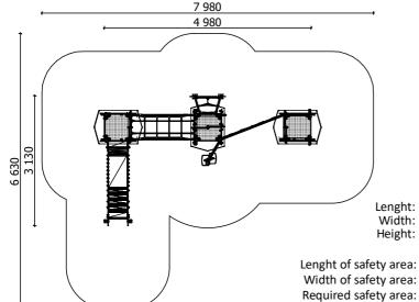
Lenght: 4 980 mm Width: 3 130 mm Height: 2 785 mm
