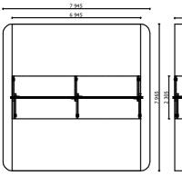
Lenght: 6 945 mm Width: 2 305 mm Height: 2 600 mm
