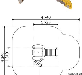
Lenght: 1 735 mm Width: 1 310 mm Height: 2 075 mm Lenght of safety area: 4 740 mm Width of safety area: 4 340 mm 16,14 m<sup>2</sup> Required safety area: (Install shock absorbing material according to EN 1176:2017)
