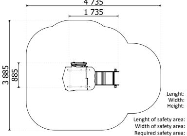
Lenght: 1 735 mm Width: 885 mm Height: 2 075 mm 4 735 mm 3 885 mm 15,12 m<sup>2</sup> (Install shock absorbing material according to EN 1176:2017)
