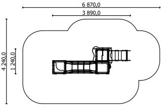
3 890 mm Lenght: Width: 1 240 mm Height: 2 150 mm
