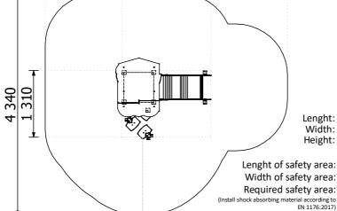
Lenght: 1 735 mm Width: 1 310 mm Height: 2 075 mm
