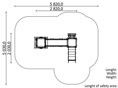
Lenght: Width: 2 820 mm 2 030 mm Height: 1 980 mm 5 820 mm 5 030 mm Width of safety area: 25 m<sup>2</sup> Required safety area: (Install shock absorbing material according to EN 1176:2017)
