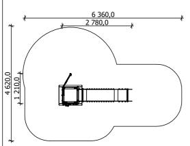
Lenght: 2 780 mm Width: 1 210 mm Height: 2 780 mm
