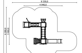
Lenght: 4 940 mm Width: 3 460 mm Height: 2 780 mm
