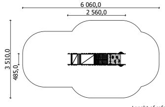
Lenght: 2 560 mm Width: 485 mm Height: 1 610 mm
