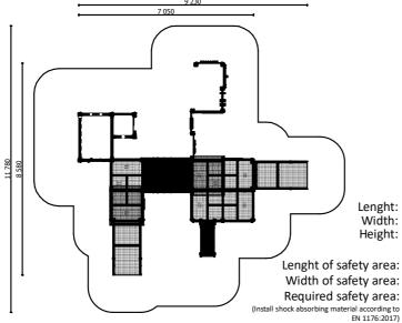
Lenght: 9 230 mm Width: 8 580 mm Height: 2 380 mm
