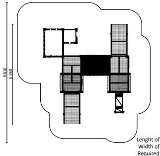
Lenght: 5 835 mm Width: 6 860 mm Height: 2 650 mm
