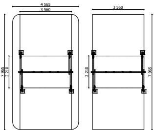
Lenght of safety area: 4 565mm Width of safety area: 7 965 mm Required safety area: 36,13 m² (Install shock absorbing material according to EN 1176:2017)
