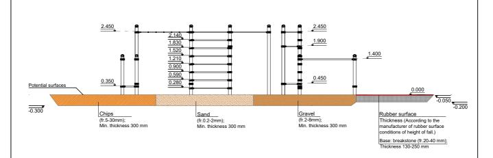
Surface type and its thickness must comply with EN 1177 standard requirements taking into account the fall height of the equipment.
