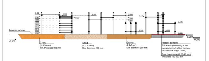
Surface type and its thickness must comply with EN 1177 standard requirements taking into account the fall height of the equipment.
