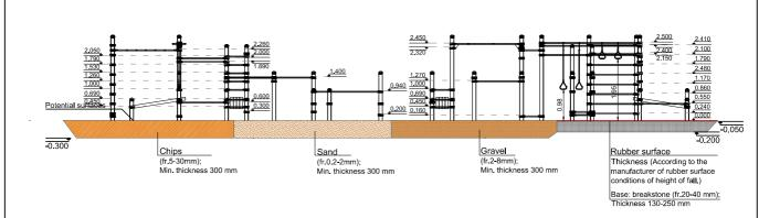
Surface type and its thickness must comply with EN 1177 standard requirements taking into account the fall height of the equipment.
