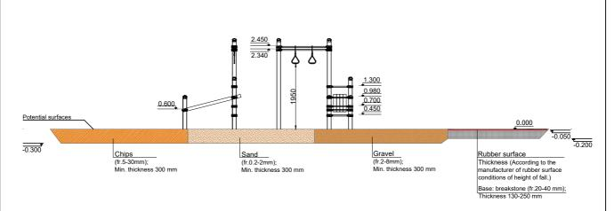
Surface type and its thickness must comply with EN 1177 standard requirements taking into account the fall height of the equipment.
