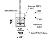
Gymnastic equipment is stablished by concreting the steel foundation in planned equipment location. Equipment is suitable for use after two days of concreting when the foundation is totally solid. During assembly no children are allowed in the area.
