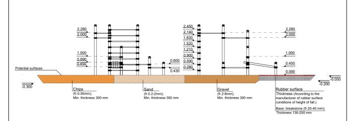
Surface type and its thickness must comply with EN 1177 standard requirements taking into account the fall height of the equipment.
