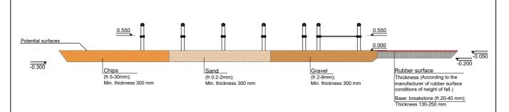
Surface type and its thickness must comply with EN 1177 standard requirements taking into account the fall height of the equipment.
