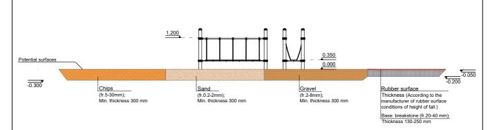
Surface type and its thickness must comply with EN 1177 standard requirements taking into account the fall height of the equipment.
