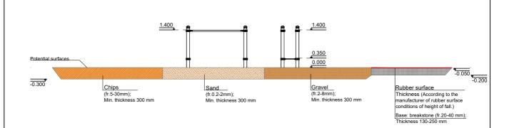
Surface type and its thickness must comply with EN 1177 standard requirements taking into account the fall height of the equipment.
